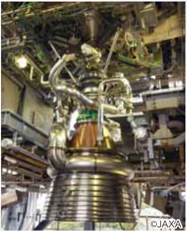
At Tanegashima Space Center LE-9 engine set on a combustion test stand EKK turbopump seals are installed on the LE-9, the first stage engine under development for the H3, the next National Flagship Launch Vehicle.
