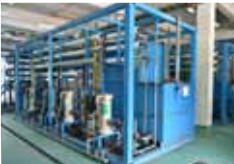
Chemical (pressure flotation) + physical (membrane purification) system
